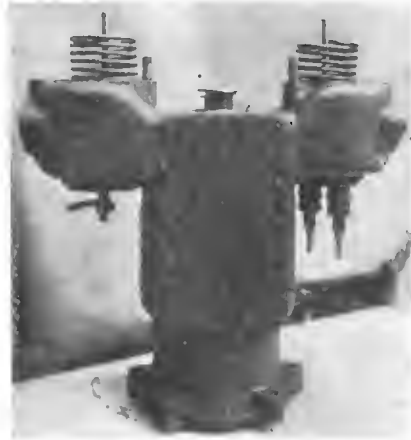
CYLINDER CASTING AND VALVE ASSEMBLY.
